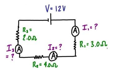
3) What is the potential difference supplied by the power source in this circuit?
