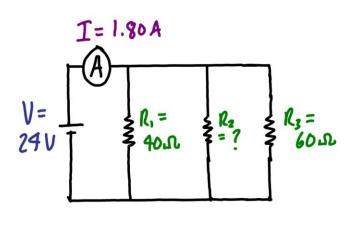
4) What are the values of  $V_1$ ,  $V_2$ , and  $R_2$  in the circuit?
