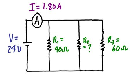
3) What is the potential difference supplied by the power source in this circuit?
