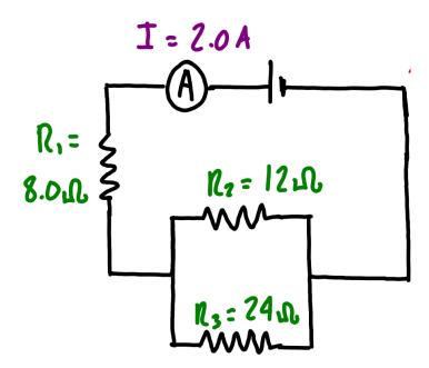
4) What are the values of  $V_1$ ,  $V_2$ , and  $R_2$  in the circuit?
