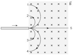
One type of ion is observed to follow path 2. Which path describes the one taken by an oppositely charged ion with twice the mass and twice the charge? (Assume all ions have the same speed.)
