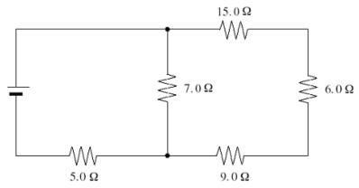
Name: \_\_\_\_\_ In Class Assignment 4) What is the total power dissipated by the three resistors in the circuit shown below? (4 marks)
