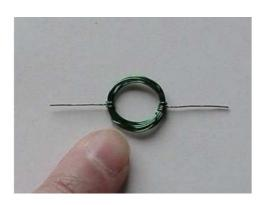
Now wrap the ends back around the coil. This will both support the coil and create the "axle" for your motor. This is the most challenging part of the experiment....
